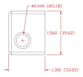
ALL DIMENSIONS GIVEN AS: in [mm] MOLDED PARTS: ±.030" [±0.8mm] HARDWARE ITEMS: ±.010" [±0.25mm]
