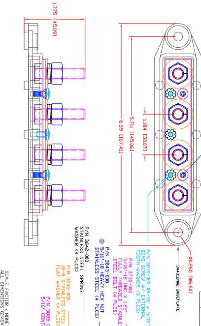
P/N 3843-008 5/16"-18 HEAVY HEX NUT STAINLESS STEEL (4 PLCS) 5/16\*-18 UNC X 1.25\* — FULLY THREADED STAINLESS STEEL BOLT (4 PLCS)
