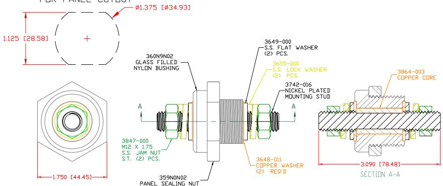
MAXIMUM FASTENER TORQUES: JAM NUTS: 198 IN-LBS [22,30 Nm] SEALING NUT: 120 IN-LBS [13.56 Nm]
