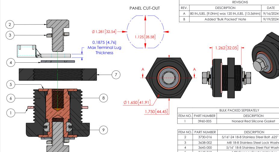
QTY. **DESCRIPTION** 5/16"-24 18-8 Stainless Steel Bolt .625" Long 2 M8 18-8 Stainless Steel Lock Washer 2 5/16" 18-8 Stainless Steel Flat Washer 2
