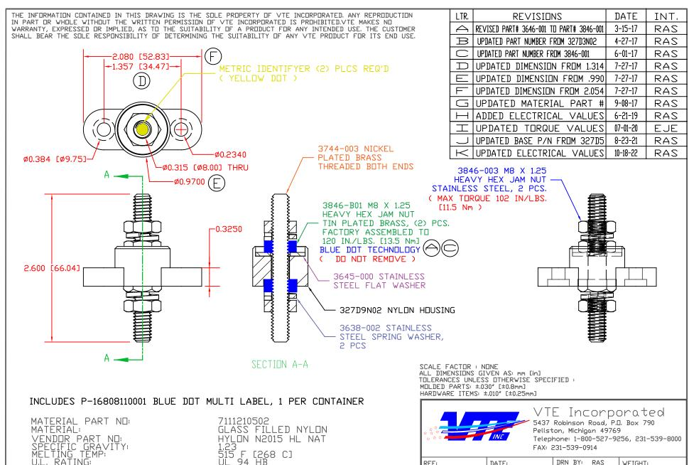
CURRENT CARRYING CAPACITY: (325 AMP @ 12VDC)
